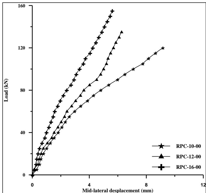
Figure (11): Load – displacement curve for RPC columns without steel fibers.
