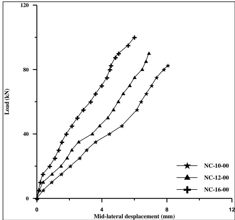
Figure (10): Load – displacement curve for normal concrete columns.
