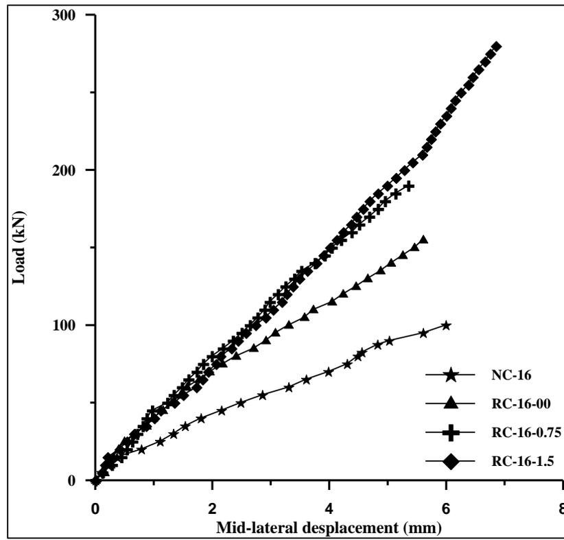
**Figure (16):** Load – displacement curve for columns with variable steel fibers content.
