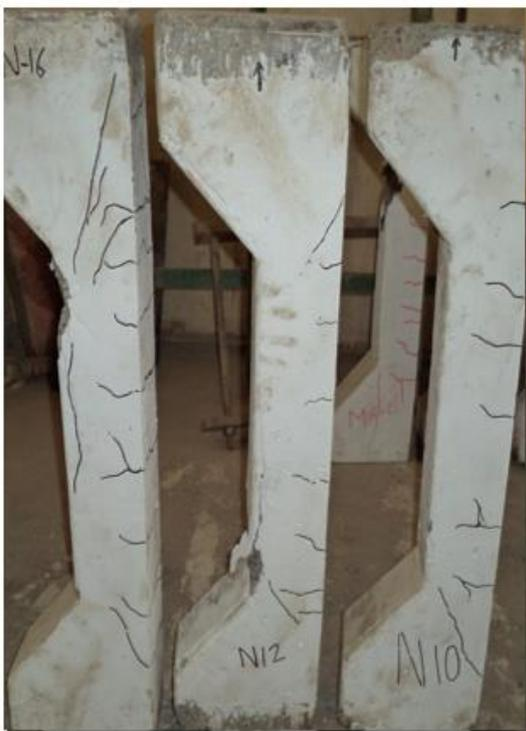
**Figure (5):** Modes of failure and crack patterns for normal concrete columns.
