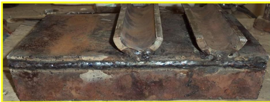
**Figure (3):** Loading cap with two grooves for eccentricity distance.
