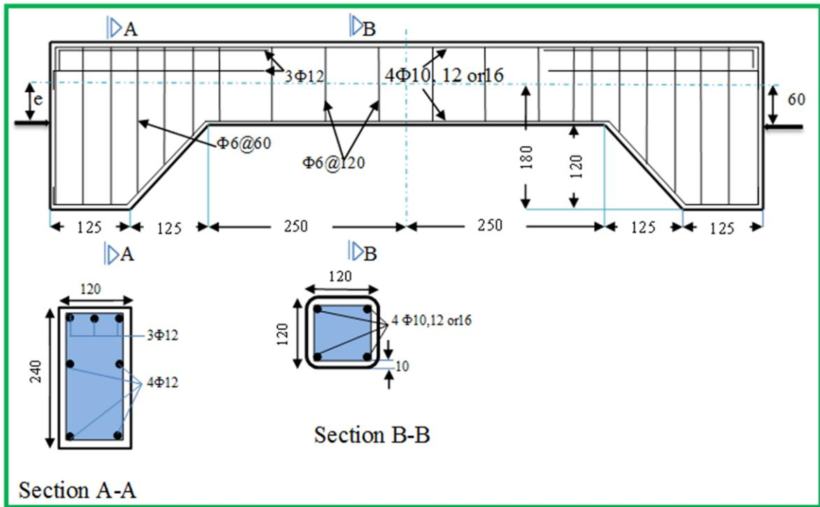
**Figure (1):** Details of specimen (All dimensions in mm).
