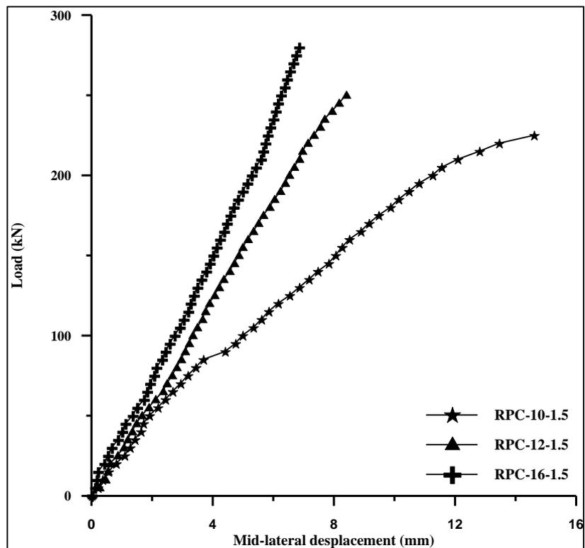
Figure (13): Load – displacement curve for RPC columns with steel fibers of 1.5%.
