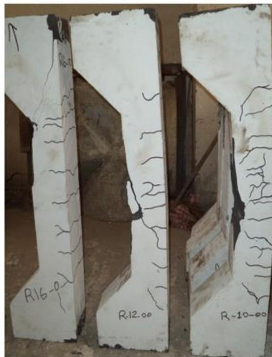
**Figure (6):** Modes of failure and crack patterns for RPC columns without steel fiber.
