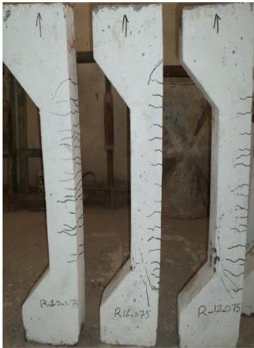
**Figure (7):** Modes of failure and crack patterns for RPC with 0.75% steel fibers.
