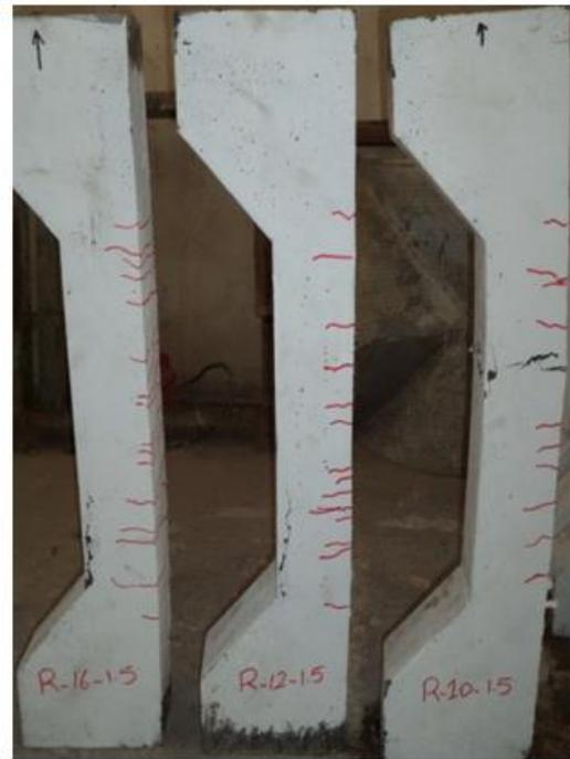
**Figure (8):** Modes of failure and crack patterns for RPC with 1.5% steel fibers.
