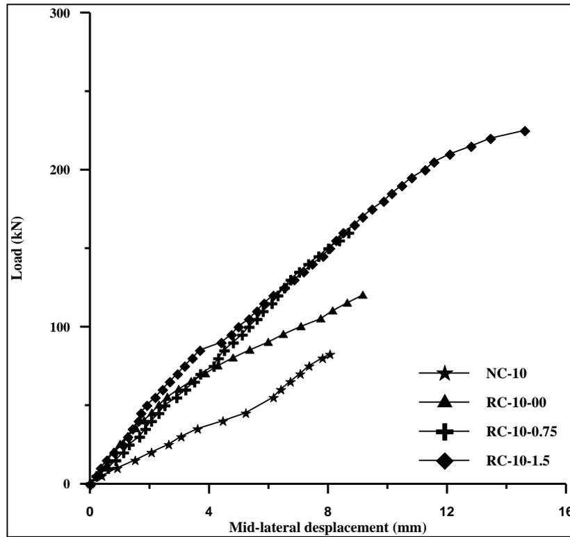
Figure (14): Load – displacement curve for columns with variable steel fibers content.
