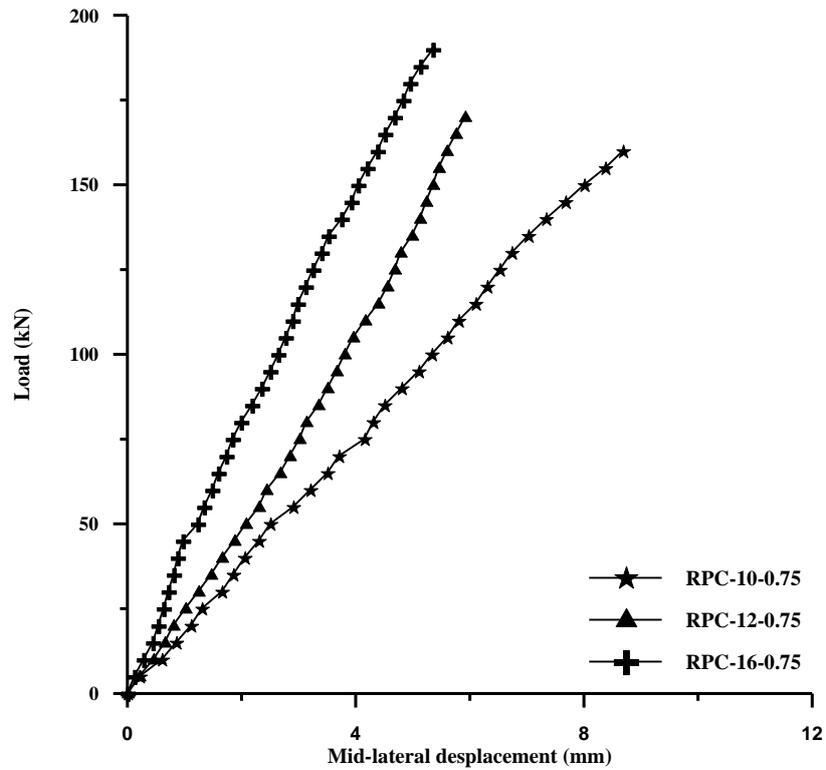
Figure (12): Load – displacement curve for RPC columns with steel fibers of 0.75%.
