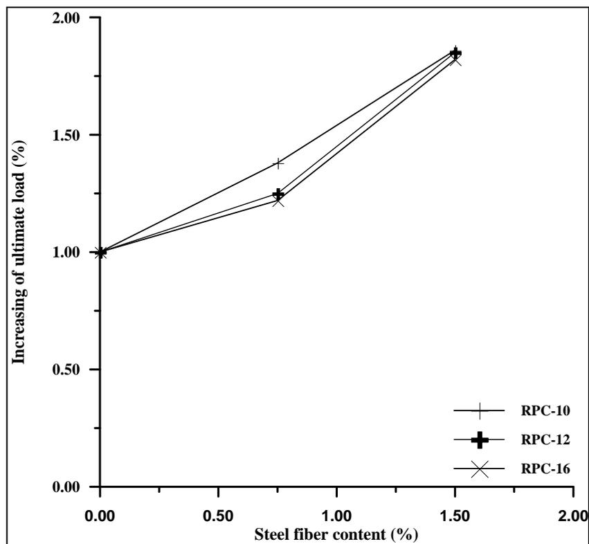
**Figure (9):** Relationship between steel fibers content and increasing in ultimate
