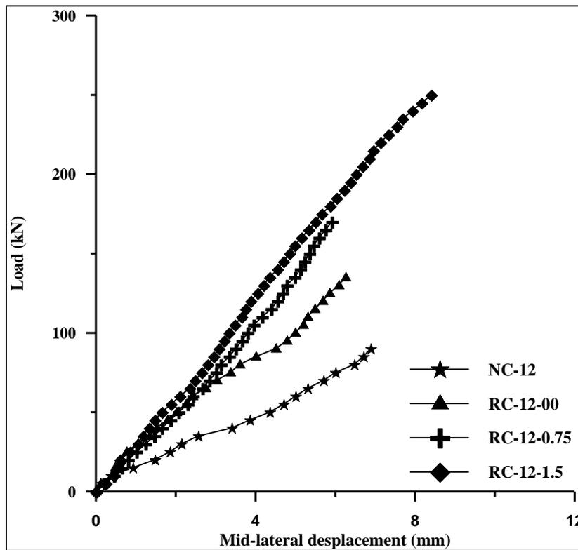
Figure (15): Load – displacement curve for columns with variable steel fibers content.
