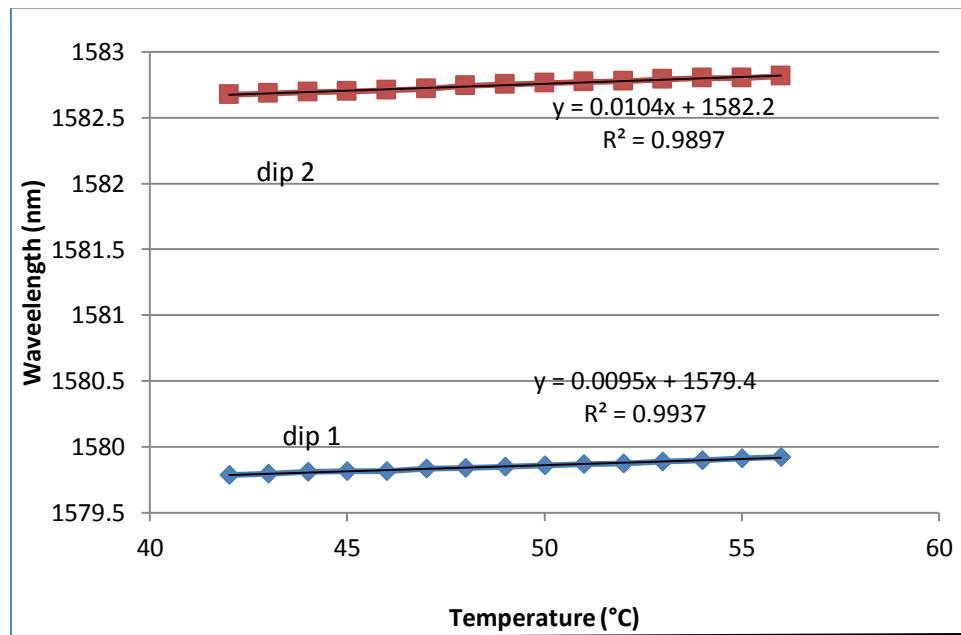
**Figure (4):** The relationship between temperature and wavelength of the first TFBG
