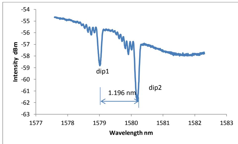
**Figure (3):** Transmission spectrum of the TFBG written on 26 cm side hole fiber.
