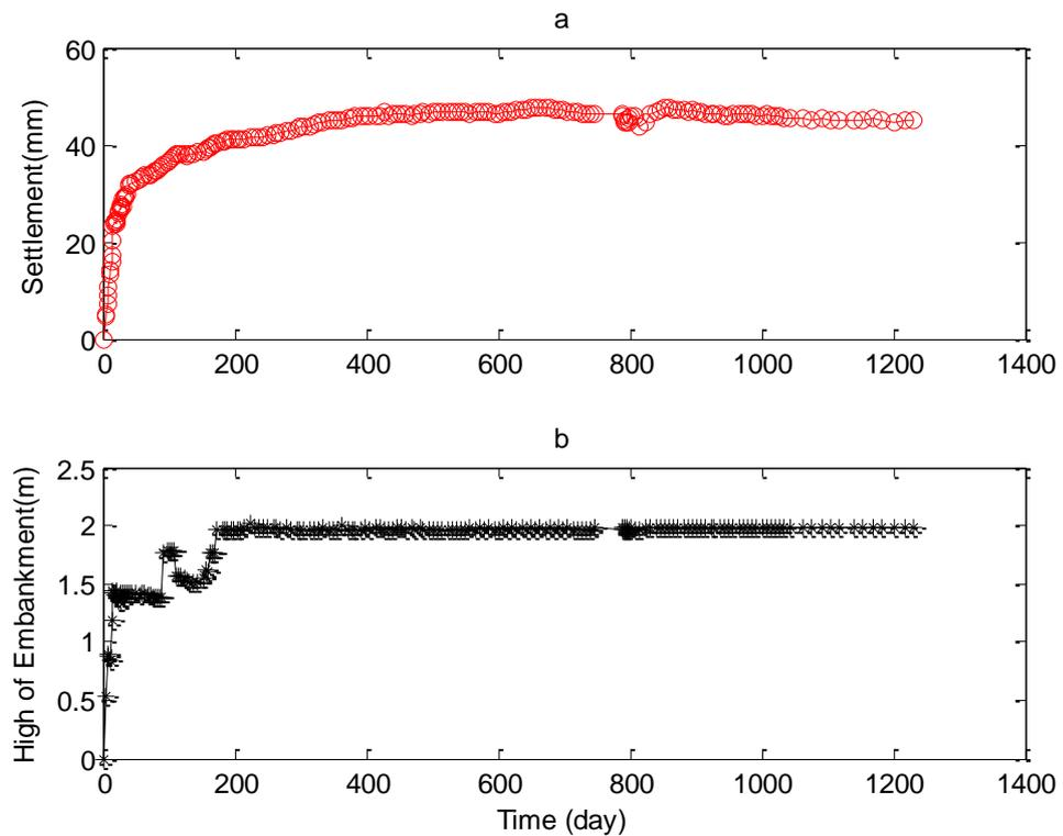
Figure 2 Stone columns behaviour under embankment: (a) settlement vs. time, (b) Relationship between
