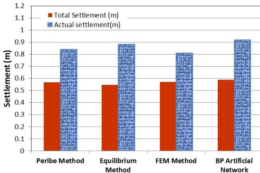
Figure 4. Compare various settlement methods of stone columns under embankment
