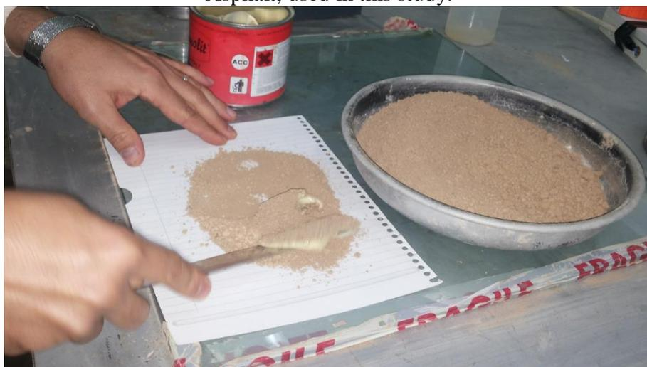
Fig (5): Preparation of sand stabilizing layer, mixed with fly ash and Polyester.
