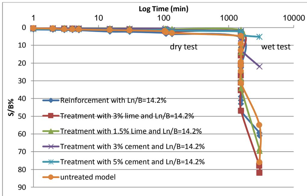
Fig (11): Stabilization of saline soil using layer of sand, mix with two additives (Cement, Lime), and 14.2% of waste ferrous materials.
