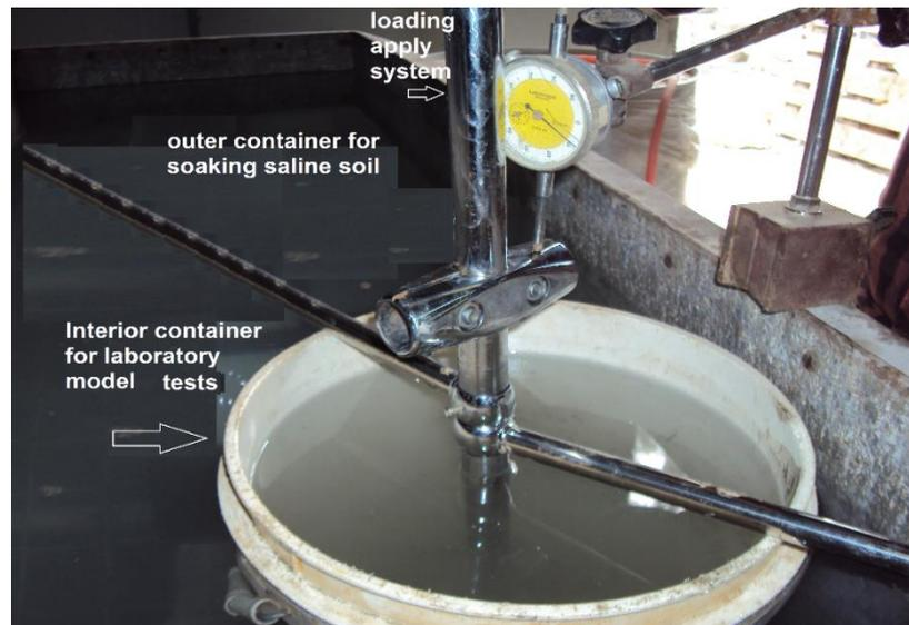
Fig. (3): Model preparation for soaking test for stabilized and unstabilized saline soil by different techniques.
