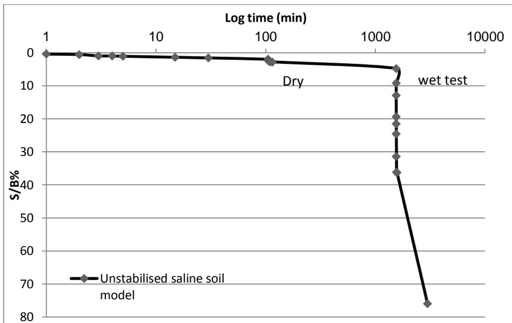
Fig (7): Results of unstabilized saline soil model for natural saline soil brought from Jurf al Milih Region in Diyala Governorate, with 10% salinity. Tested at  $36.6 \text{ kN/m}^2$  applied stress.
