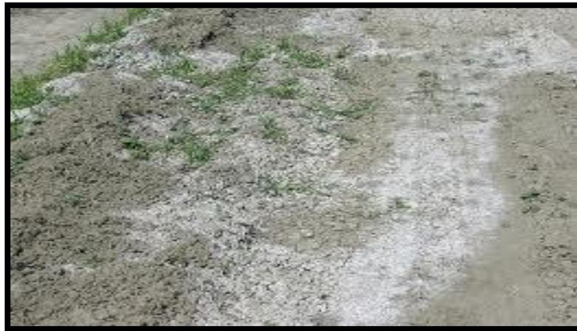
Fig. (1) Soil sample taken from a region near Jurf Al-Milih region in Diyala governorate, which extruded from 1m depth. With 10% salt percent.
