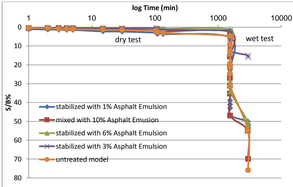
Fig (9): stabilization of saline soil by a layer of graded sand mixed with Asphalt Emulsion with different percentages (1%, 3%, 6% and 10%).
