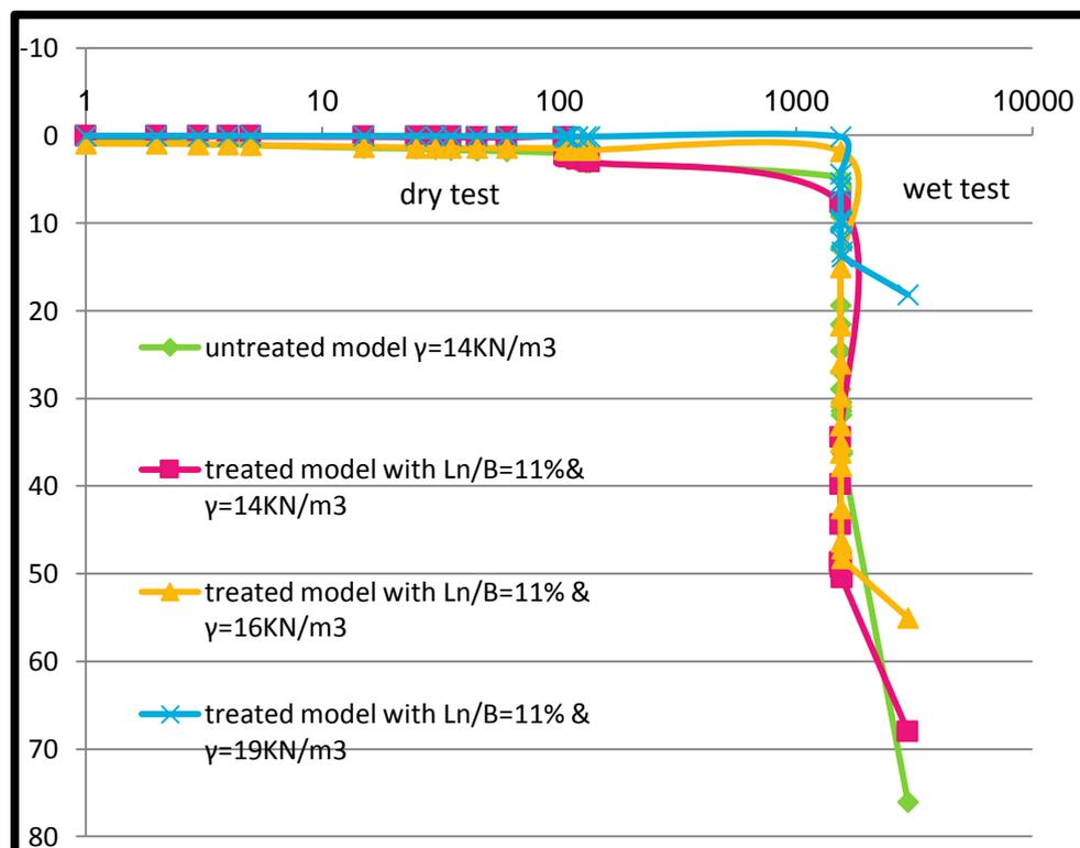
Fig (12) Stabilization of saline soil using a stabilized sand layer, by compaction and the use of 11% randomly distributed waste ferrous material.
