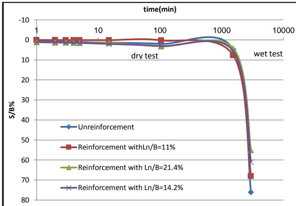
Fig (13): Stabilization of saline soil using a layer of sand with the addition of randomly distributed waste ferrous materials (11%, 14.2% and 21.4%)
