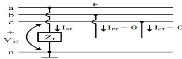
Figure 3 General representation of a single line-to-ground fault.
