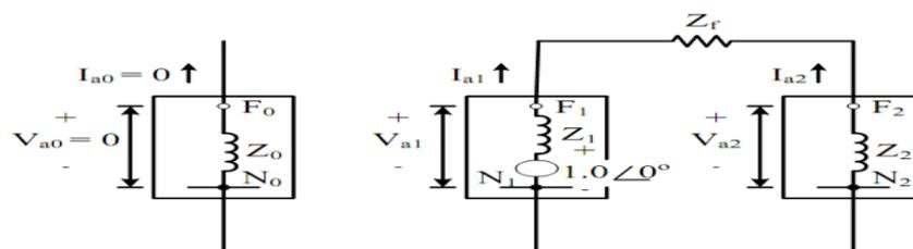
Figure 7 Sequence network diagram of a line-to-line fault.
