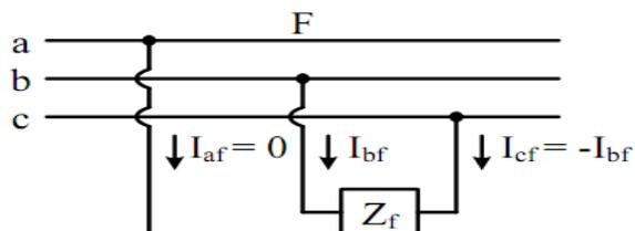
Figure 6 Sequence network diagram of a line-to-line fault
