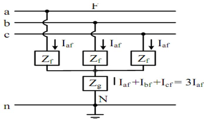
Figure 12 General representation of a balanced three-phase fault
