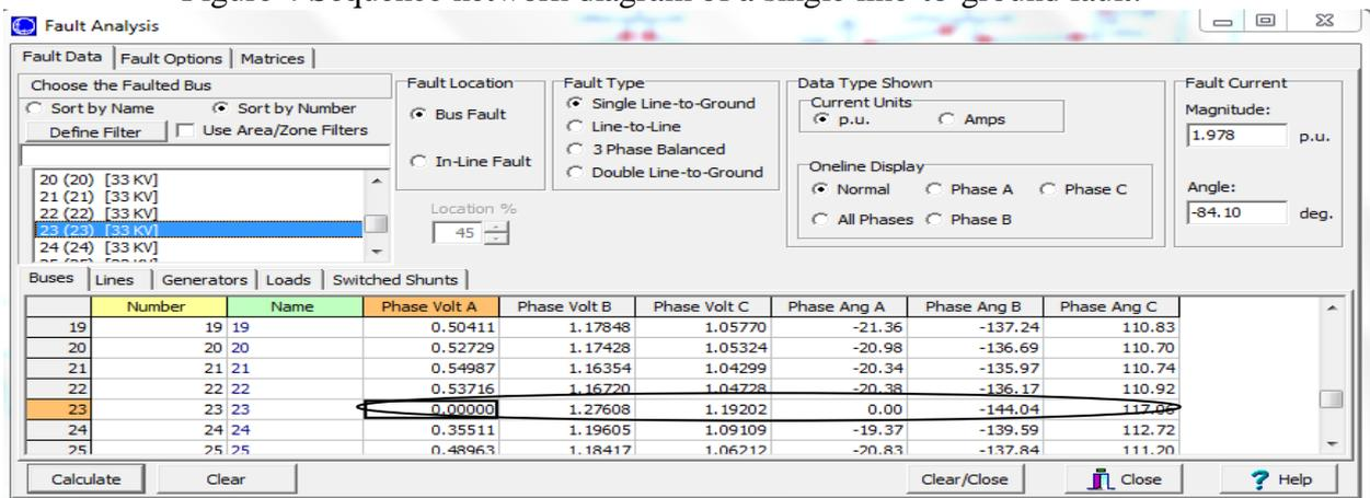
Figure 5 show power world simulators to calculate fault current the type single line to ground.
