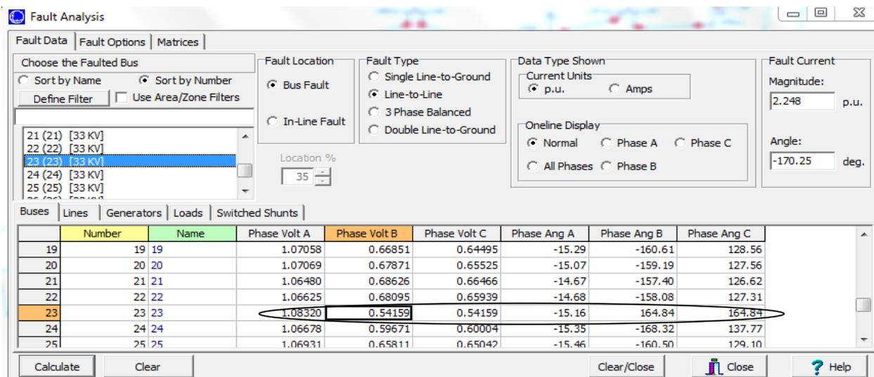
figure 8 show using power world program to calculate current in the type fault line to line
