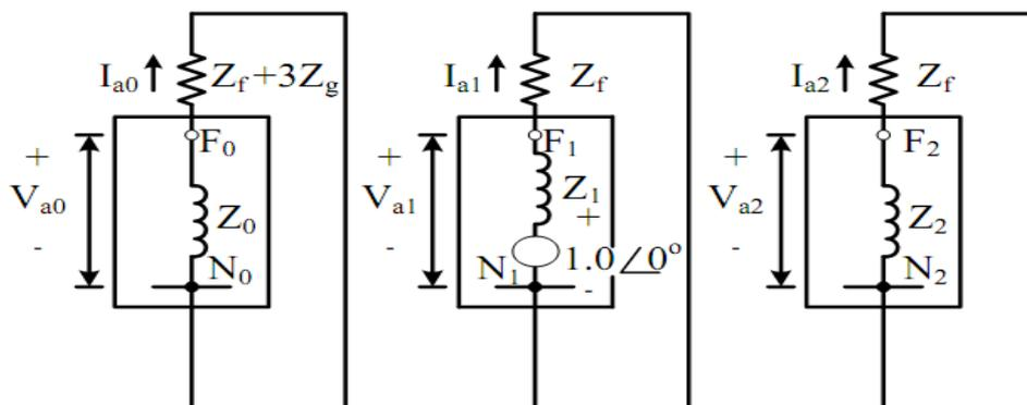
Figure 13 Sequence network diagram of a balanced three-phase fault
