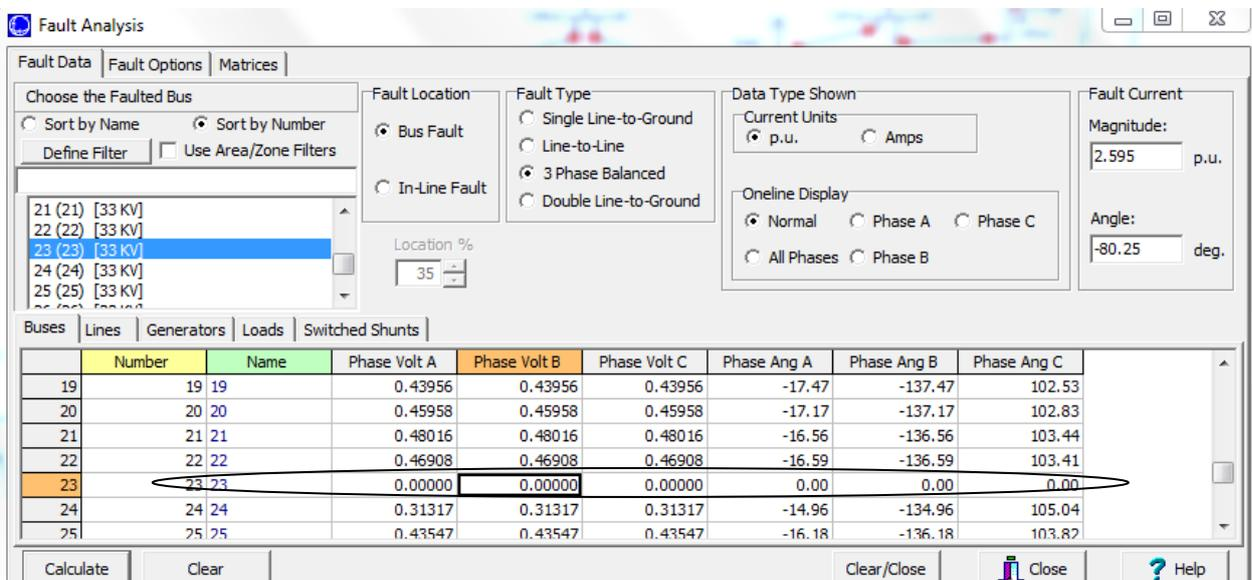
Figure 14 show using power world program to calculate current in the type fault three phase
