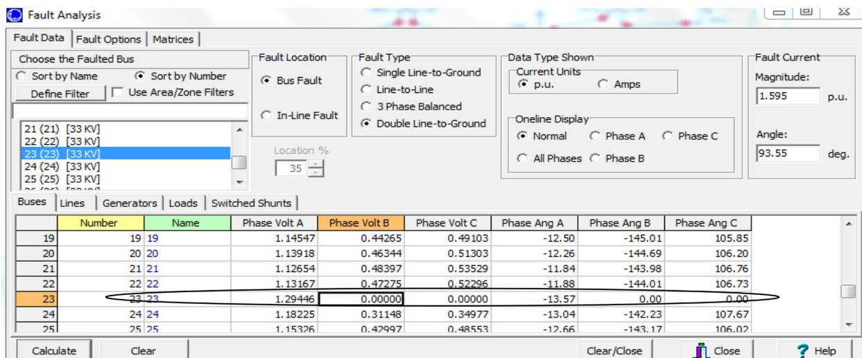
figure 11 show using power world program to calculate current in the type fault double line
