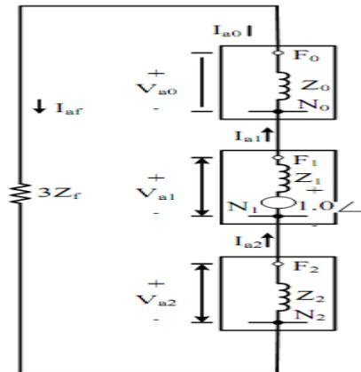
Figure 4 Sequence network diagram of a single line-to-ground fault.
