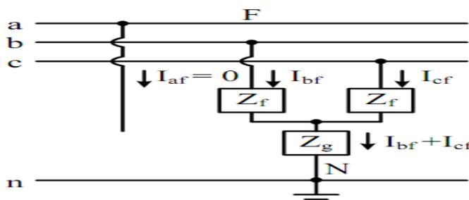
Figure 9 General representation of a double line-to-ground fault.
