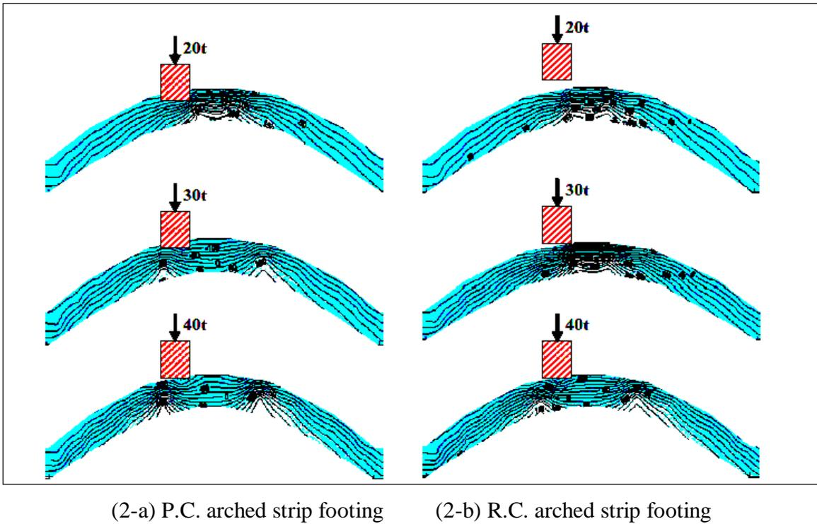
**Fig. 2.** Effect of load increasing on the normal stress ( $s_x$ ) contour in R.C. & P.C arched strip footing at ratio  $(t/B) = 0.1$ ,  $(h/B) = 0.2$  and silty clay soil.
