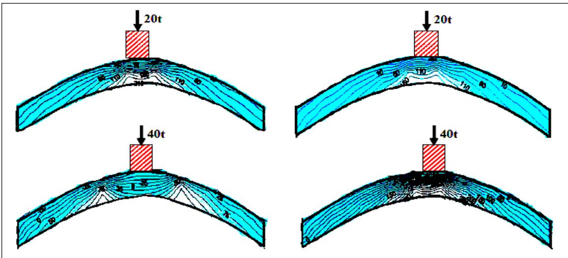
**Fig. 3.** Effect of load increasing on the normal stress ( $s_x$ ) contour in R.C. & P.C arched strip footing at ratio  $(t/B) = 0.1$ ,  $(h/B) = 0.2$  and silty sand soil.
