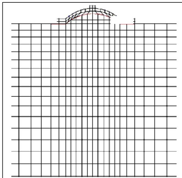
(1-a)Proposed finite-infinite element mesh
